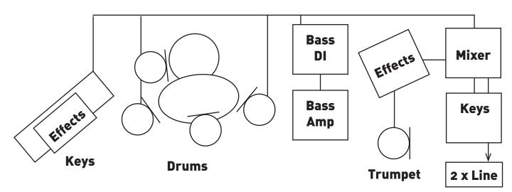
On small stages Wolkenpark delivers a fully mixed signal in stereo and uses in-ear monitoring. On big stages the band needs at least 2 monitor lines (keys/tp, dr/b) with 3 monitors.
